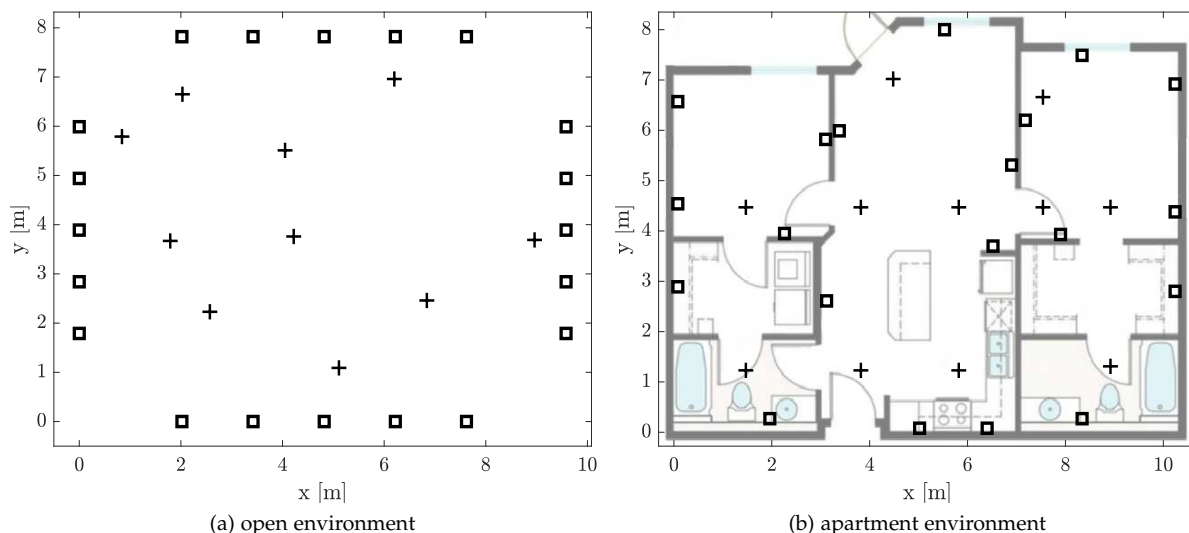
Fig. 4: The experimental layouts in which the nodes ( \square ) and the validation positions ( + ) are illustrated. The apartment was fully furnished with two beds, nightstands, cupboards, a sofa, coffee table, etc., but the furniture is omitted from the figure.
