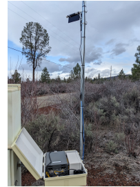
Fig. 7. Our RDZ test transmitter in a weatherproof junction box stalled at HCRO.
