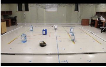
(a) The lab setup with obstacles, moving node, and PVC pipes as boundary.
