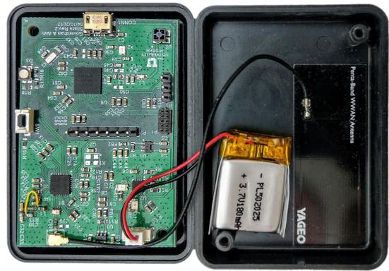
Fig. 1: *Sitara* PCB with antenna and rechargeable battery housed in an ABS plastic enclosure
