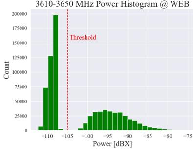
Fig. 2: Power Level Histogram at 3610-3650 MHz
